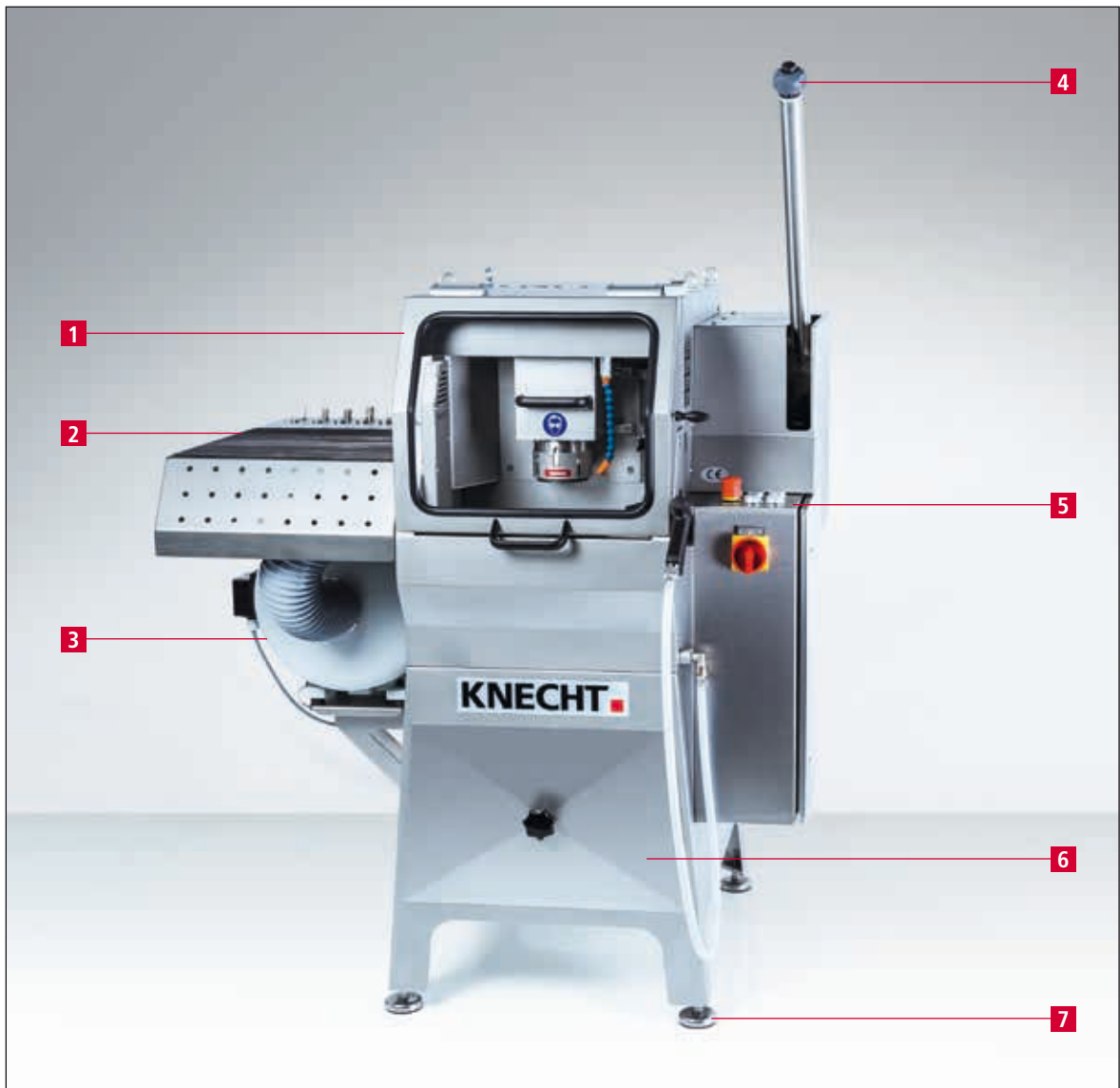
Figure 3-2 General view of grinding machine
