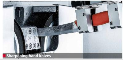
Perfectly ground hand knives enable more accurate cuts. Hand knives, ground with the E 50 R robotic technology, increase the yield of meat up to 0,5 % compared to manual grinding. At 10 000 tons meat production, this means a 50 000 kilograms higher rate of yield.
