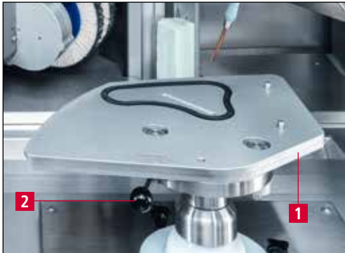
Figure 7-6 Fixing the knife holder
