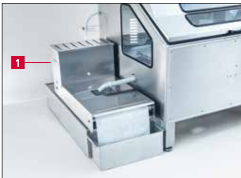
Figure 6-1 Belt filter coolant unit
