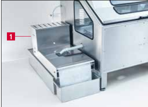
Figure 3-8 Belt filter coolant unit
