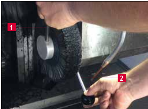
Figure 7-15 Changing the finned brushes of the polishing unit
