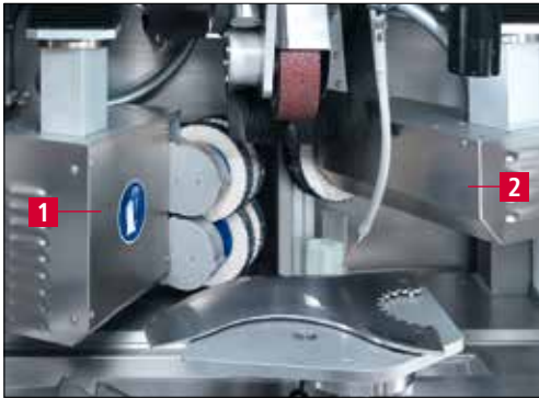
Figure 3-16 Polishing units with polishing paste
