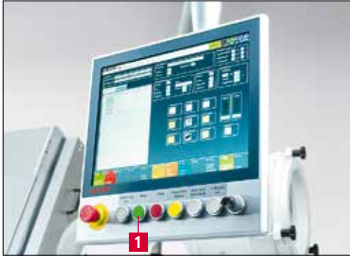
Figure 7-9 Starting the grinding program
