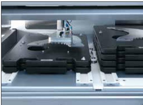
Figure 3-17 Knife magazine with knife changer
