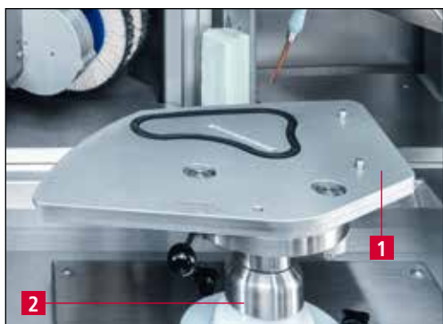
Figure 7-5 Placing the SP 114 knife holder
