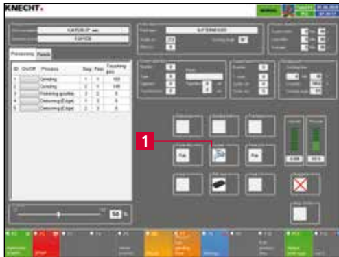
Figure 9-3 Switching the coolant pump On/Off
