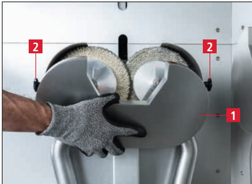
Figure 7-18 Removing the protection hood
