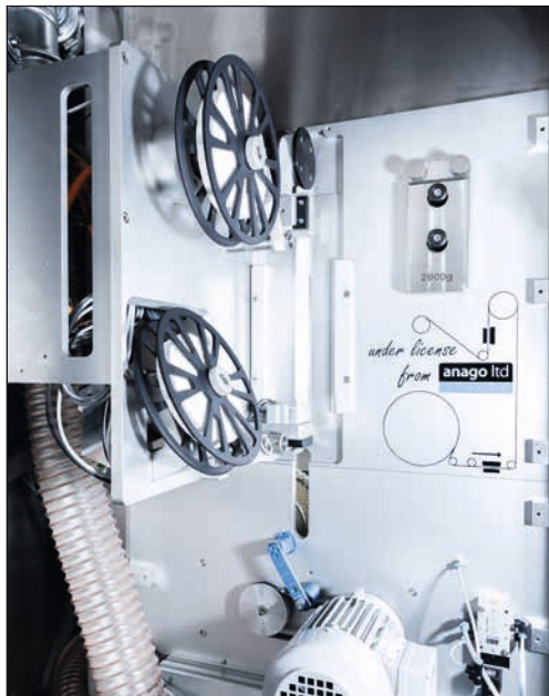
Figure 7-22 Opening the sharpness testing device
