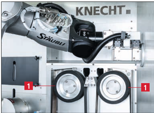
Figure 7-7 Replacing the wet-grinding belt
