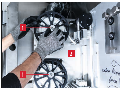
Figure 7-23 Removing the test medium
