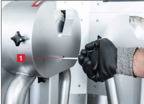
Figure 7-21 Setting the polishing/deburring rings
