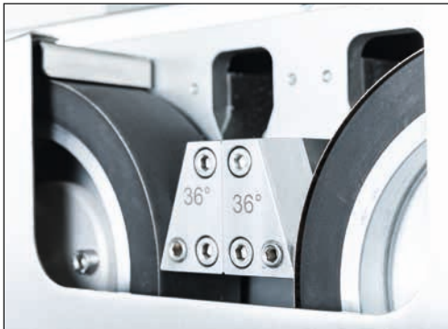
Figure 7-11 Adjusting the wet-grinding belt
