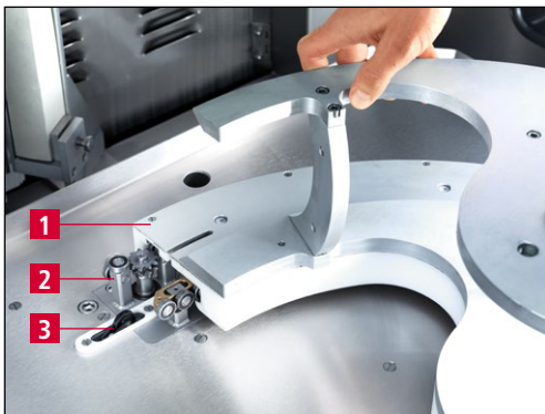
Figure 7-2 Mounting the copy grinding plate
