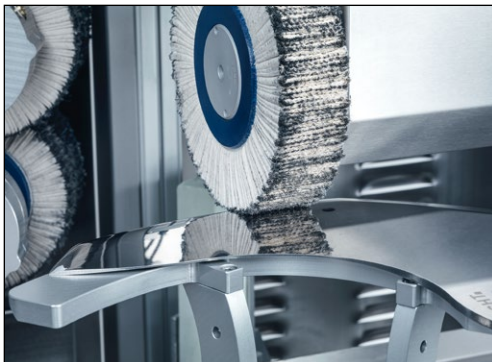
Figure 7-12 Aligning the polishing unit
