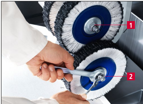
Figure 7-22 Changing the finned brushes of the deburring unit
