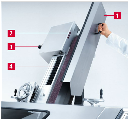
Figure 7-17 Changing the wet grinding belt
