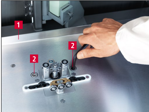
Figure 9-7 Dismantling the guard plate
