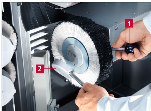
Figure 7-20 Changing the finned brush of the polishing unit
