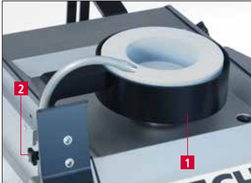
Figure 7-11 Adjusting the grinding wheel guard
