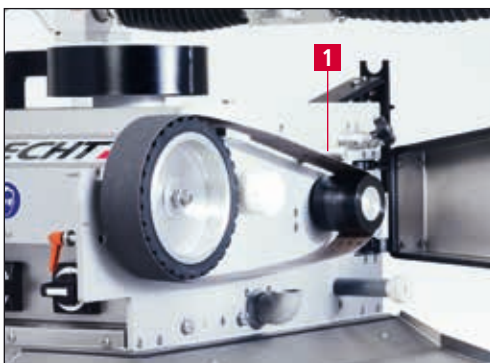
Figure 7-14 Changing the wet-grinding belt
