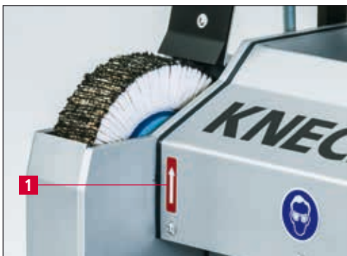
Figure 6-2 Checking the direction of rotation
