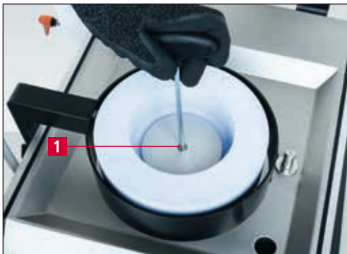
Figure 7-12 Changing the grinding wheels
