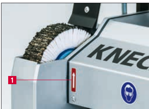
Figure 6-2 Checking the direction of rotation
