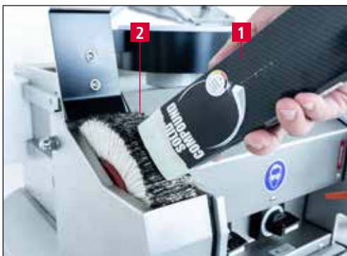
Figure 7-5 Applying the polishing paste
