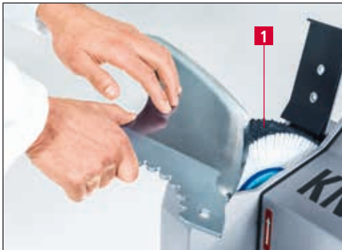
Figure 7-6 Deburring and polishing cutter knives
