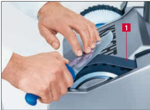
Figure 7-7 Grinding hand knives
