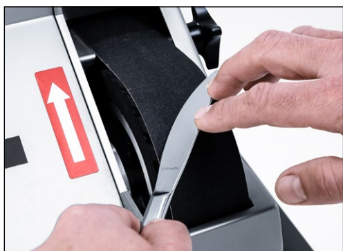
Figure 7-18 Grinding out the existing serration
