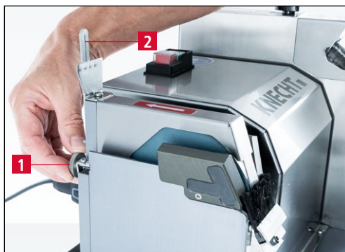
Figure 7-1 Setting the grinding angle
