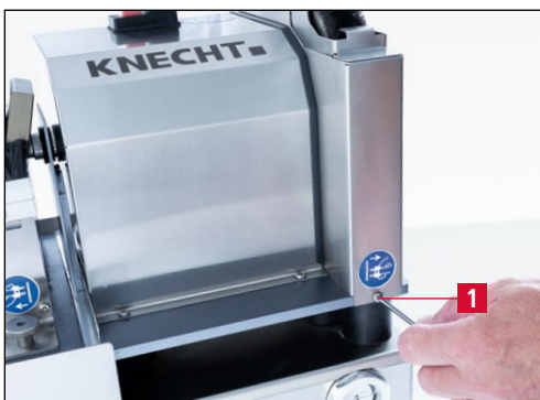
Figure 7-11 Loosening the polishing disk cover
