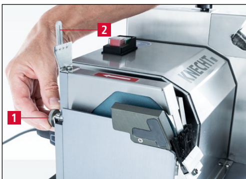
Figure 7-1 Adjusting the grinding angle
