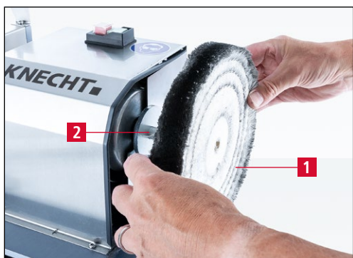
Figure 7-14 Replacing the polishing disk
