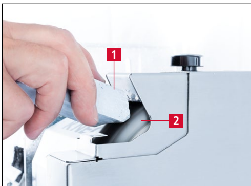
Figure 7-4 Applying the polishing paste
