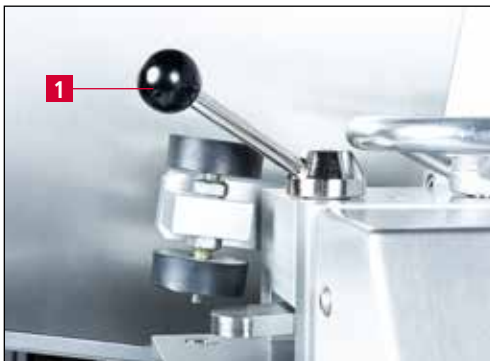
Figure 7-1 Moving the copy grinding device into change position
