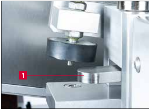
Figure 7-5 Swiveling the copy grinding device to working position
