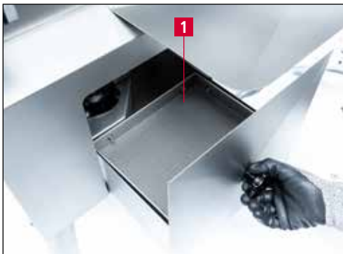
Figure 6-1 Filling the water tank
