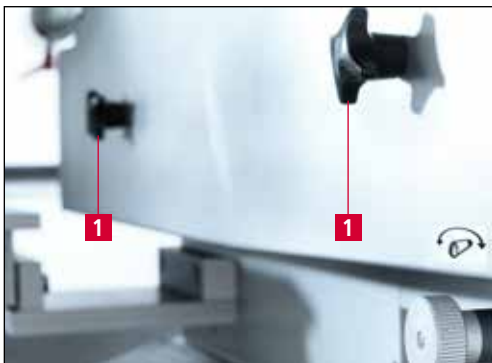
Figure 7-17 Opening the belt protection hood
