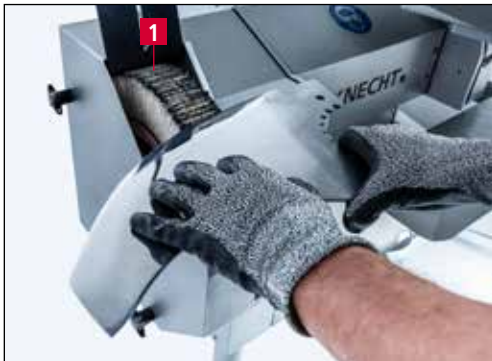
Figure 7-10 Polishing/deburring the cutter knife
