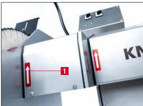
Figure 6-2 Checking the direction of rotation
