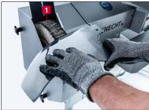
Figure 7-14 Polishing/deburring the cutter knife
