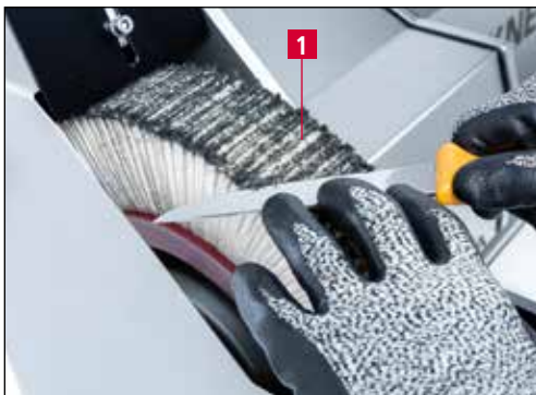
Figure 7-16 Polishing hand knives
