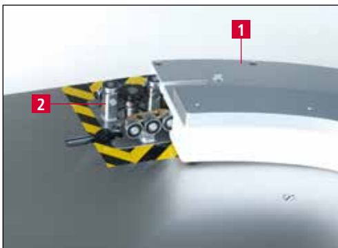
Figure 7-2 Mounting the copy grinding plate
