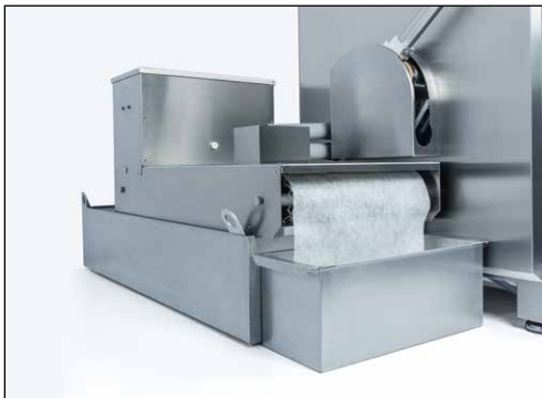
Figure 6-1 Filling the belt filter coolant unit
