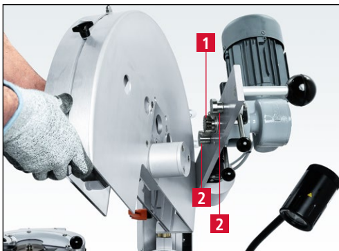
Figure 7-6 Mounting the circular knife holding fixture
