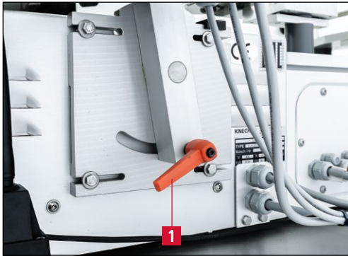
Figure 7-40 Loosening the clamping lever
