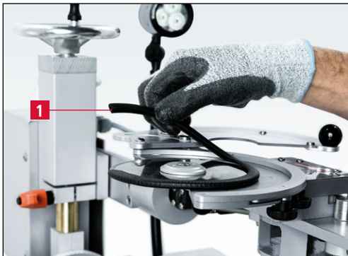
Figure 7-55 Removing cutting edge protection
