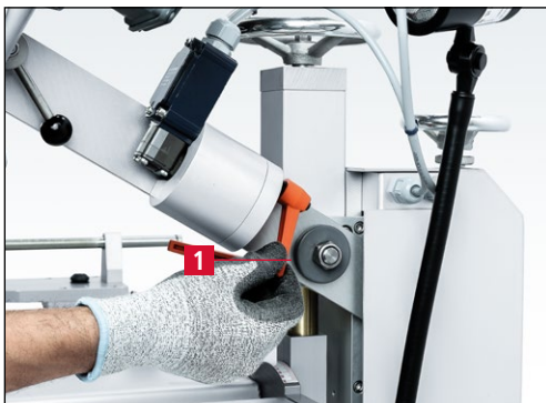
Figure 7-72 Loosening the clamping lever
