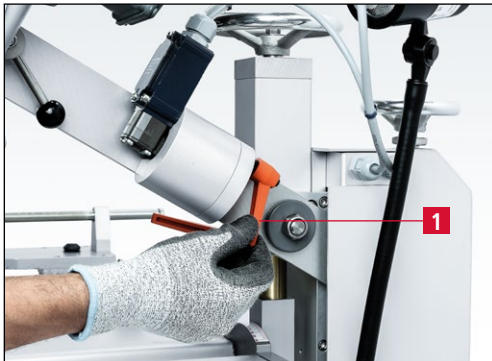
Figure 7-49 Loosening the clamping lever
