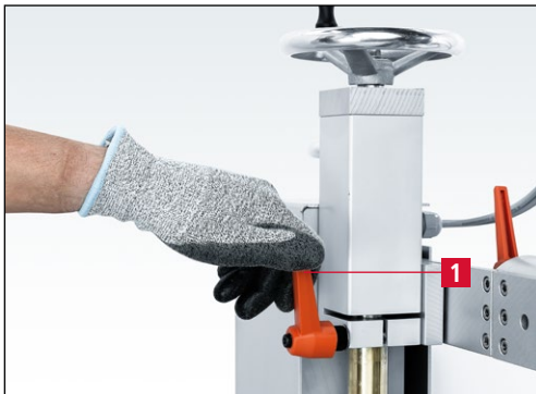
Figure 7-61 Opening the "Height adjustment" clamping lever (7-61/1).
