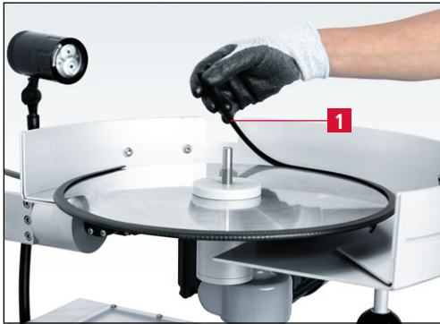
Figure 7-16 Removing cutting edge protection
