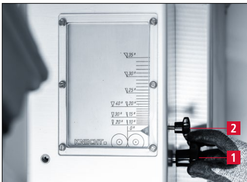
Figure 7-43 Locking the display arrow
