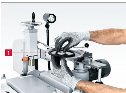
Figure 7-53 Placing the circular knife
