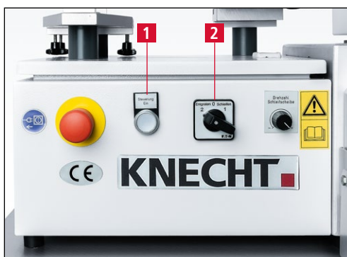
Figure 6-2 Turn on the sharpening machine
