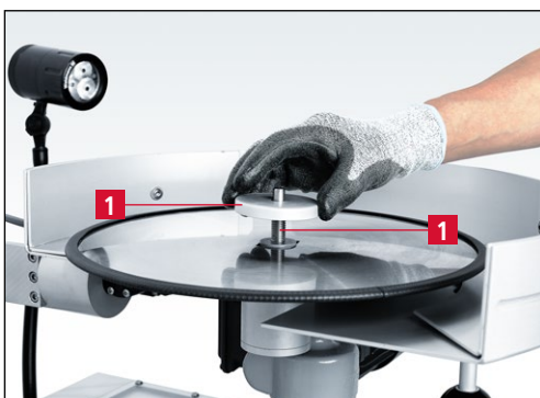
Figure 7-15 Placing the clamping flange on the locating bolt
