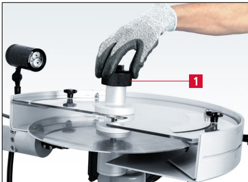
Figure 7-17 Placing the safety screen
