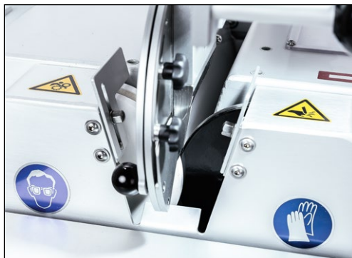
Figure 7-77 Use of the hardened steel wheel
