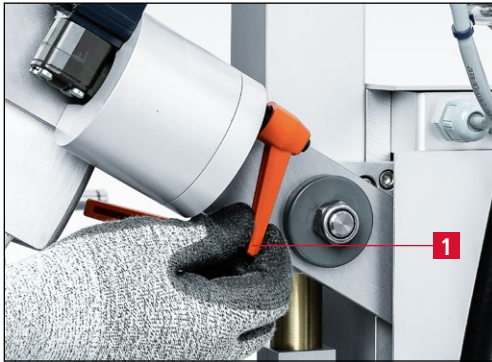
Figure 7-19 Loosening the clamping lever
