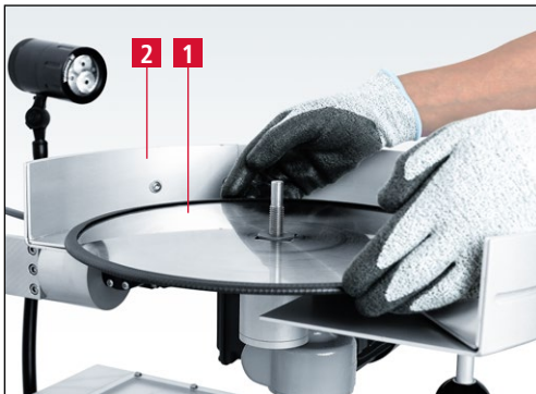
Figure 7-14 Placing circular knife on the circular knife holding fixture
