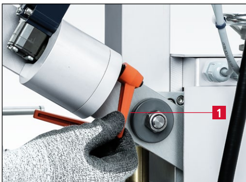
Figure 7-58 Loosening the clamping lever
