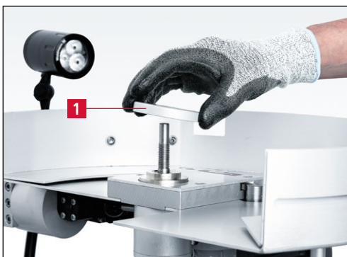
Figure 7-12 Removing clamping flange
