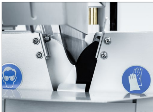
Figure 7-38 Use of the hardened steel wheel
