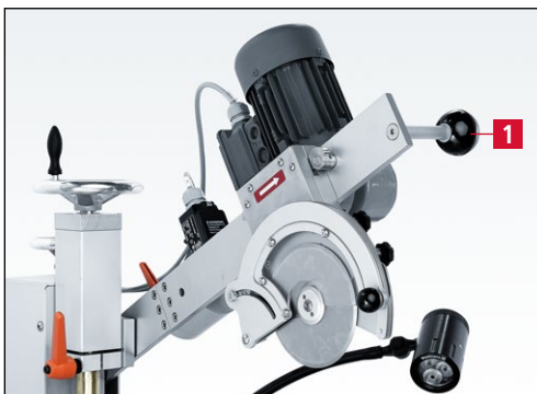
Figure 7-59 Swiveling the circular knife grinding attachment into the grinding position
