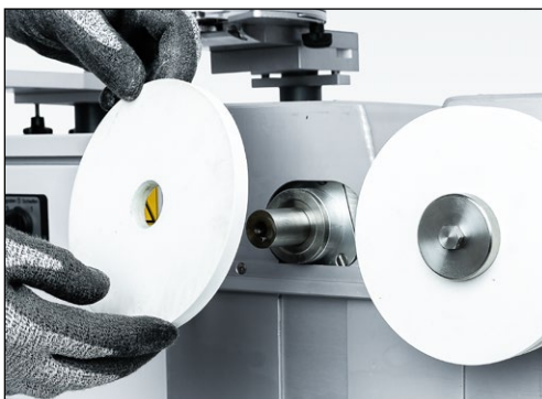
Figure 7-93 Removing grinding wheels and replacing with new ones
