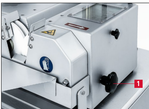
Figure 7-80 Opening the grinding wheels
