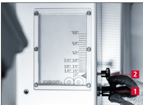
Figure 7-2 Locking the display arrow
