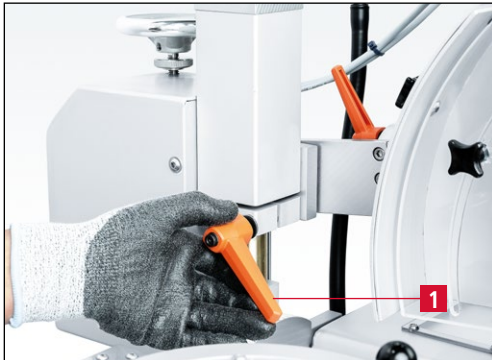
Figure 7-22 Opening the “Height adjustment” clamping lever (7-22/1).
