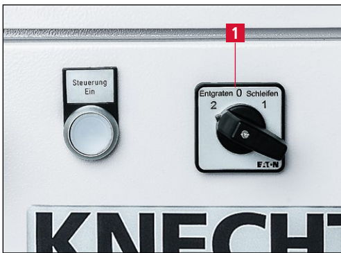
Figure 7-82 Turning on the sharpening machine
