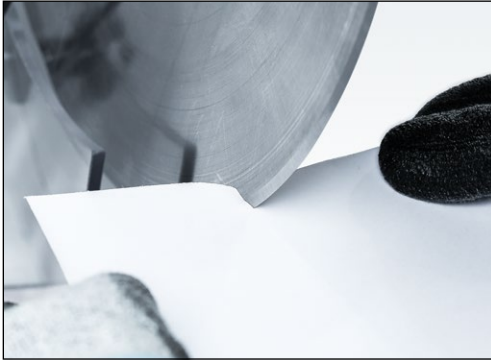
Figure 7-32 Checking the knife sharpness
