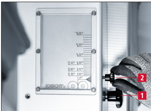
Figure 7-45 Setting the grinding angle
