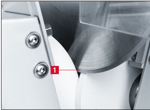
Figure 7-25 Knife moving away from the grinding wheels
