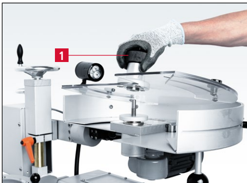
Figure 7-11 Removing clamping nut with the safety screen
