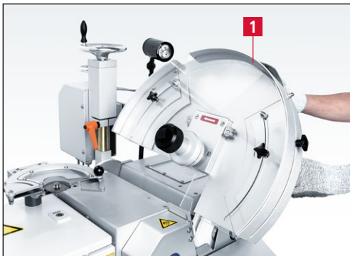
Figure 7-9 Swiveling the circular knife grinding attachment to the right
