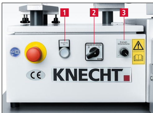
Figure 7-66 Turning on the circular knife sharpening machine
