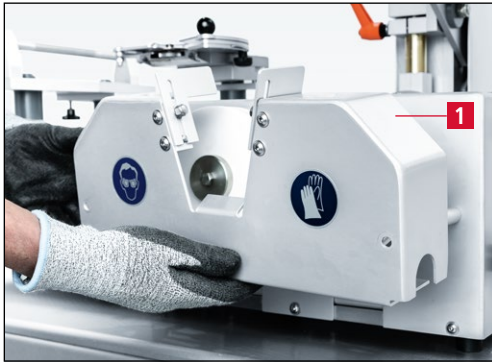
Figure 7-88 Removing the protection hood
