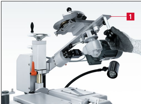
Figure 7-57 Swiveling the circular knife grinding attachment upwards
