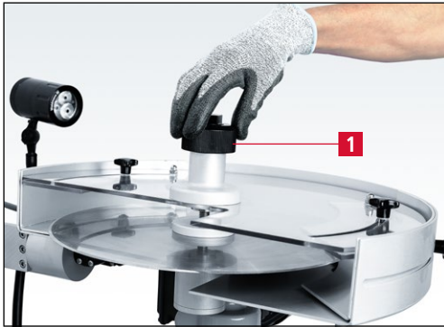
Figure 7-35 Unclamping the circular knife
