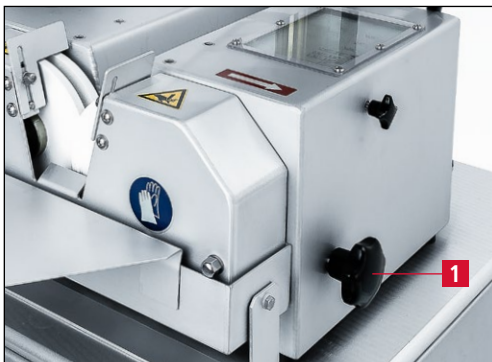
Figure 7-89 Changing position of the grinding wheels
