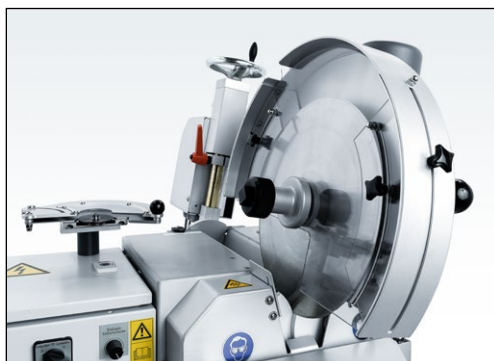
Figure 7-39 Setting the grinding unit at an angle
