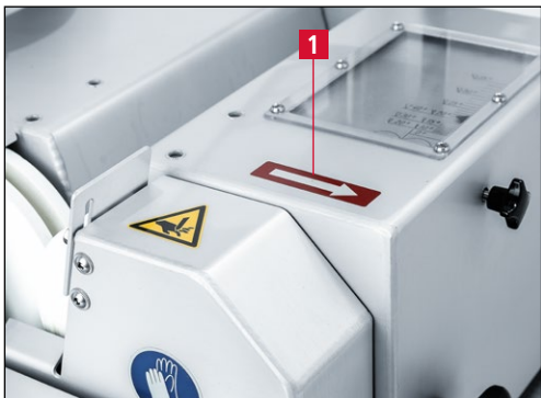
Figure 6-3 Checking the direction of rotation
