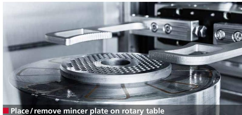
■ Place/remove mincer plate on rotary table
