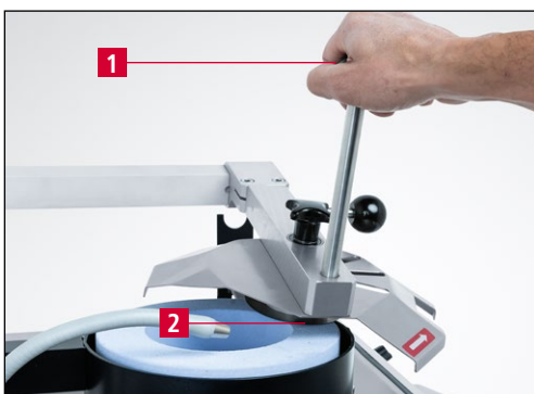
Figure 7-11 Grinding the circular knife
