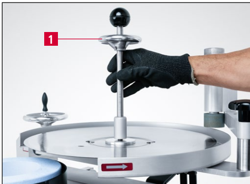
Figure 7-17 Clamping the circular knife
