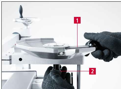
Figure 7-4 Securing the circular knife
