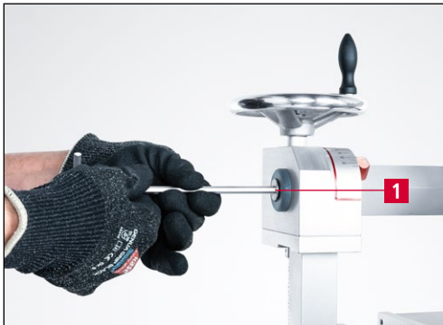
Figure 6-1 Removing the swivel arm
