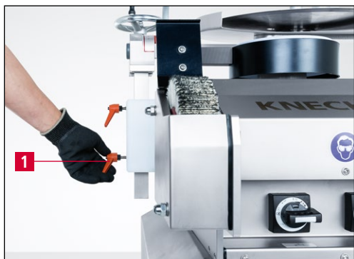
Figure 7-19 Adjusting the circular knife grinding attachment
