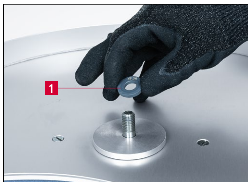
Figure 7-15 Placing the centering disk on the locating bolt
