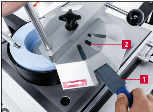
Figure 7-12 Deburring circular knives
