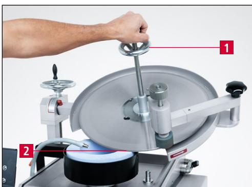
Figure 7-23 Grinding the circular knife
