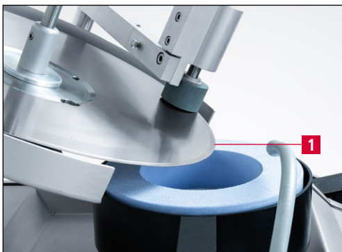
Figure 7-18 Positioning the circular knife on the grinding wheel
