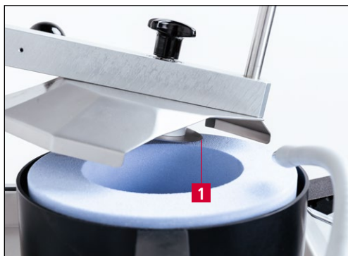
Figure 7-5 Positioning the circular knife on the grinding wheel
