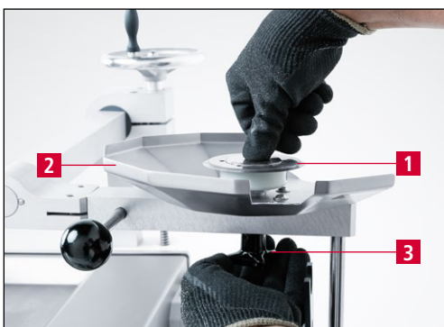
Figure 7-3 Clamping the circular knife
