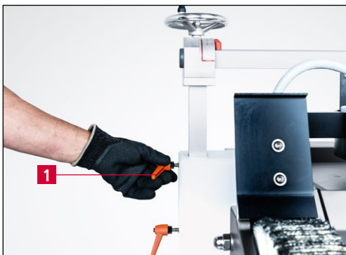
Figure 7-8 Loosening the clamping lever
