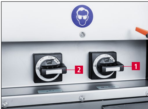
Figure 7-10 Switching on the grinding machine and coolant unit
