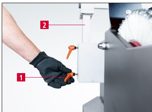
Figure 7-6 Adjusting the circular knife grinding attachment
