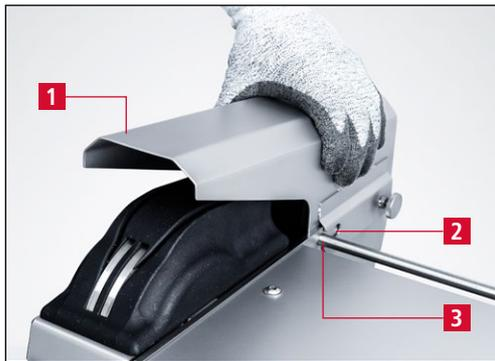
Figure 6-15 Monter le capot antiprojections
