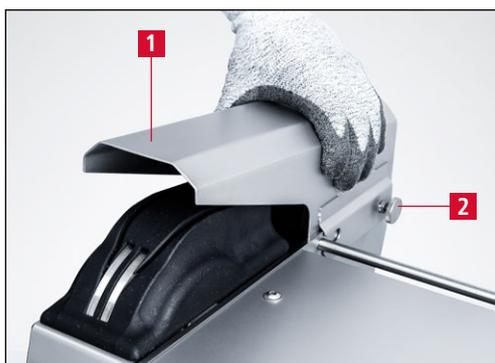
Figure 7-6 Retirer le capot antiprojections
