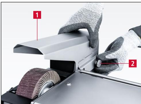
Figure 6-1 Retirer le capot antiprojections
