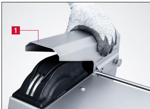
Figure 6-16 Retirer le capot antiprojections
