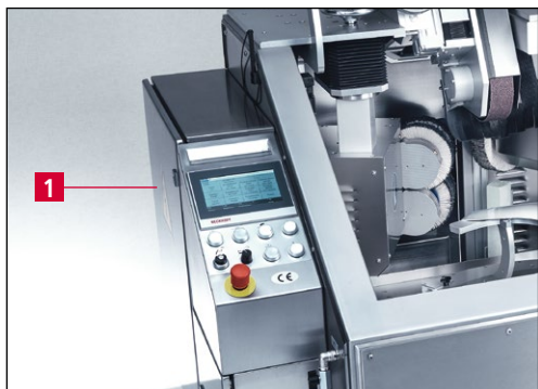
Figure 8-26 Armoire de commande
