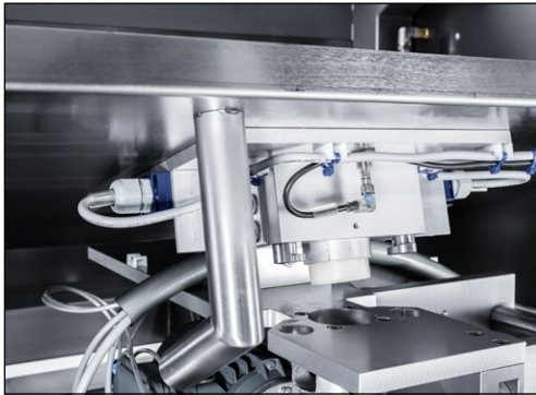
Figure 9-7 Removing the sliding plate
