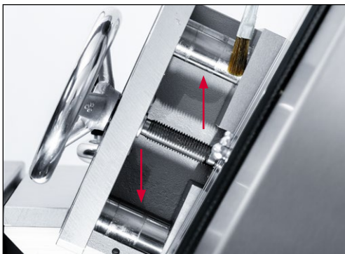
Figure 9-12 Lubricating the guides and adjustment spindle for angle setting
