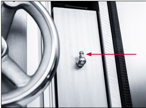
Figure 9-10 Lubricating the front of the guideway housing
