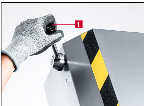
Figure 7-60 Swiveling the belt relief lever upwards
