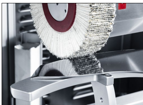
Figure 7-21 Polishing brush rests on knife
