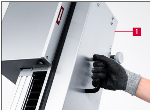
Figure 7-63 Attaching the belt protection hood
