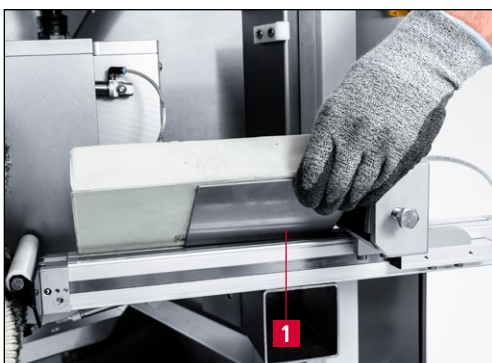
Figure 7-81 Replacing the polishing paste of the deburring unit
