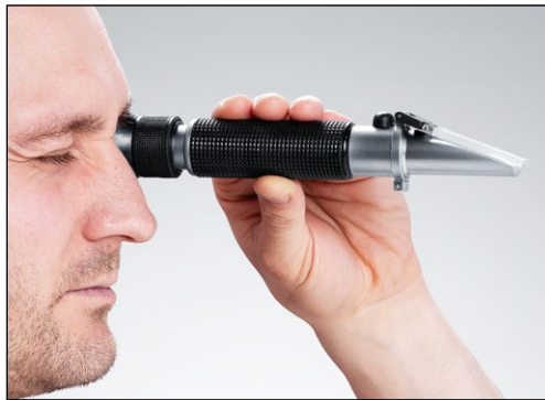
Figure 9-23 Reading the refractive index
