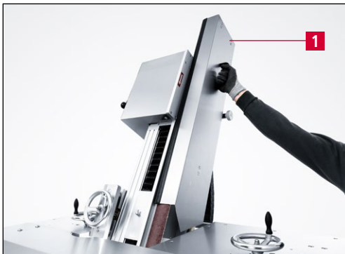
Figure 7-59 Removing the belt protection hood
