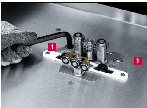
Figure 9-6 Loosening the sliding plate
