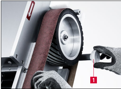
Figure 7-62 Adjusting the grinding belt run
