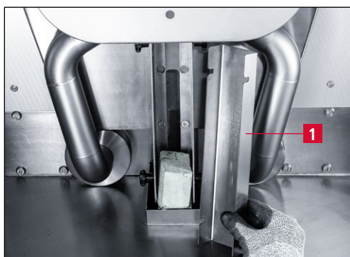
Figure 7-60 Removing the cover
