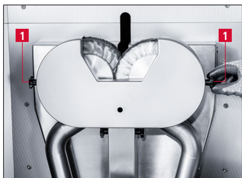
Figure 7-40 Loosening the star handles
