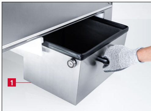
Figure 9-2 Emptying the drawer of the suction unit
