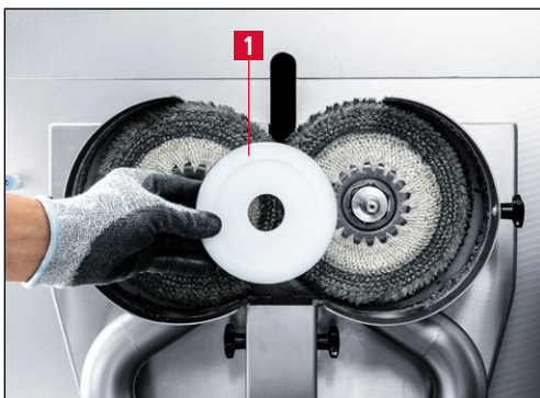
Figure 7-32 Removing intermediate flange
