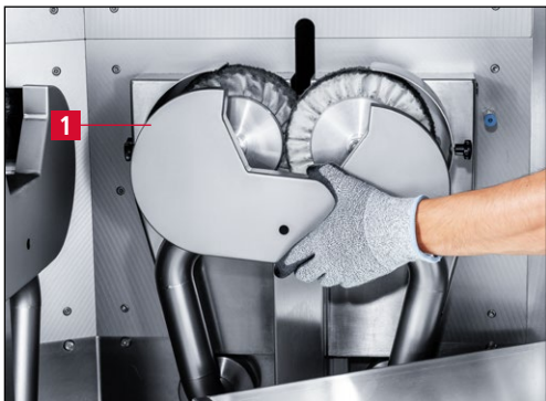
Figure 7-41 Removing the protection hood
