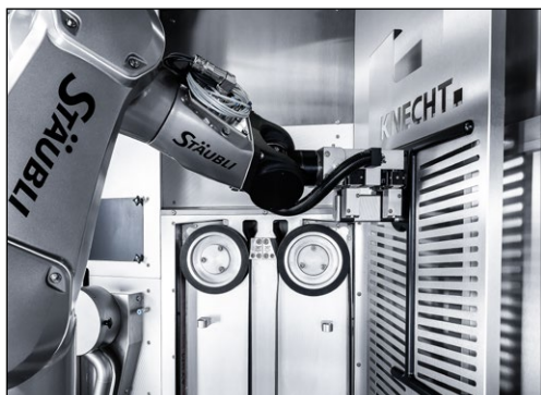
Figure 7-11 Closing the belt protection hood
