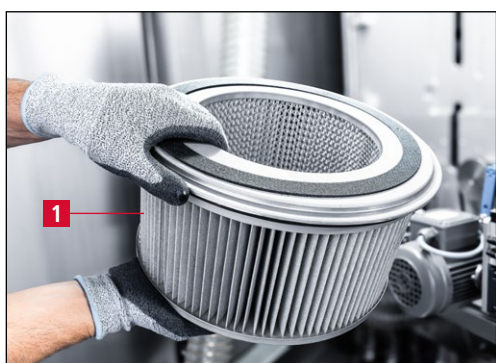
Figure 9-5 Cleaning the filter cartridge
