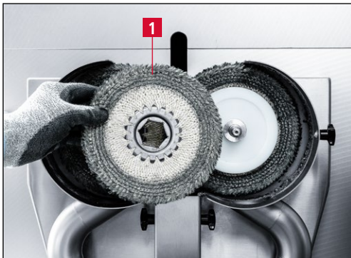
Figure 7-31 Removing the used deburring ring
