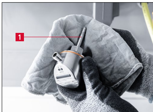
Figure 9-8 Cleaning the measuring probe
