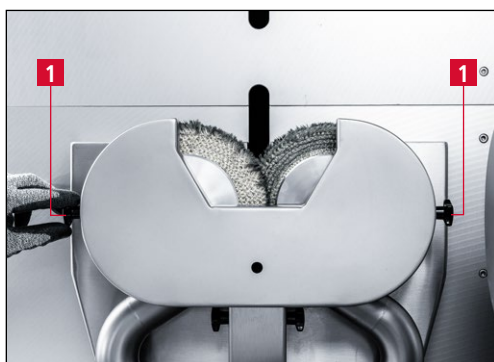
Figure 7-23 Loosening the star handles
