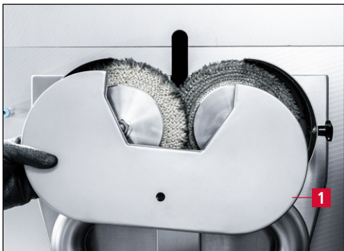
Figure 7-24 Removing the protection hood
