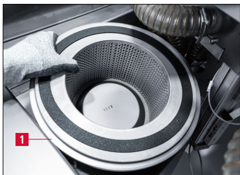
Figure 9-4 Removing the filter cartridge
