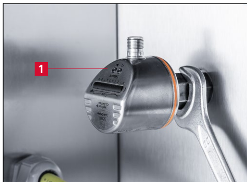
Figure 9-7 Unscrewing the flow monitor
