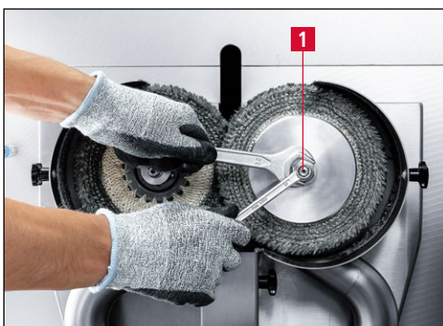
Figure 7-29 Unscrewing the right clamping nut
