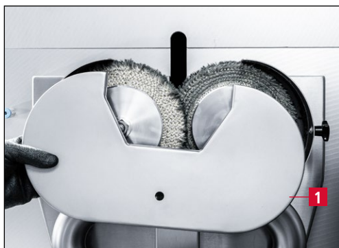
Figure 7-22 Removing the protection hood
