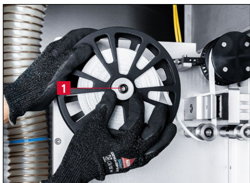
Figure 7-63 Removing the used test medium
