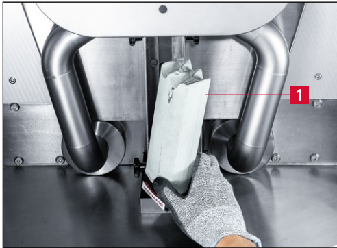
Figure 7-61 Replacing the polishing paste
