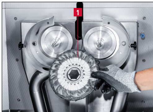
Figure 7-51 Replacing the polishing rings
