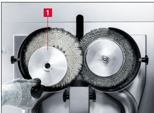
Figure 7-26 Removing the flange washer
