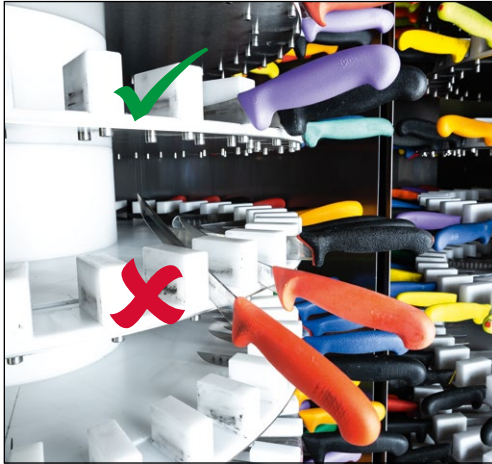
Figure 7-5 Placing the knife
