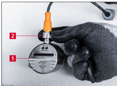
Figure 9-6 Unplugging the flow monitor
