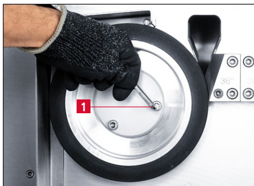
Figure 9-11 Removing the contact discs
