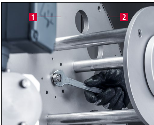
Figure 7-5 Mounting the SP 116 Cam plate
