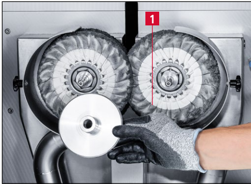
Figure 7-45 Removing the flange washer (7-45/1).
