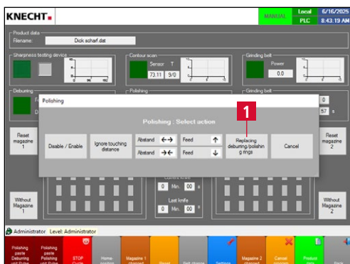
Figure 7-37 Polishing – Changing the polishing rings
