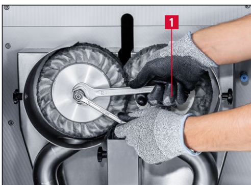
Figure 7-44 Unscrewing the left clamping nut
