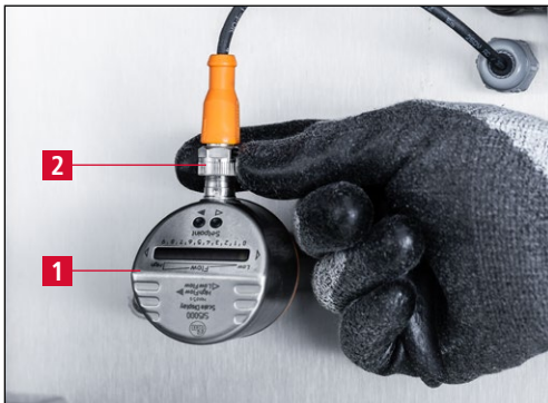
Figure 9-6 Unplugging the flow monitor
