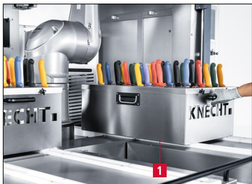
Figure 7-3 Moving the knife magazines into the grinding machine
