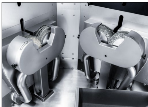
Figure 3-4 Deburring and polishing units
