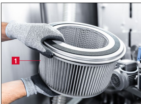
Bild 9-5 Cleaning the filter cartridge
