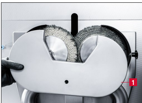
Figure 7-22 Removing the protection hood
