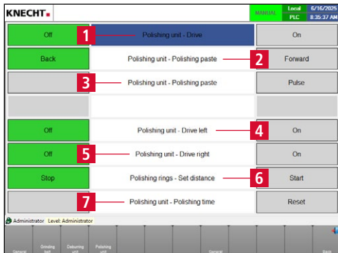
Figure 8-11 Manual functions “Polishing unit”
