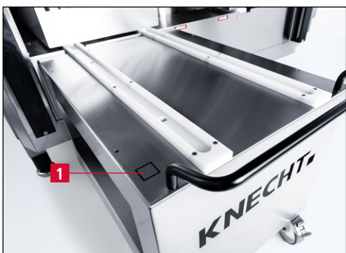
Figure 5-3 Markings on magazine trolleys
