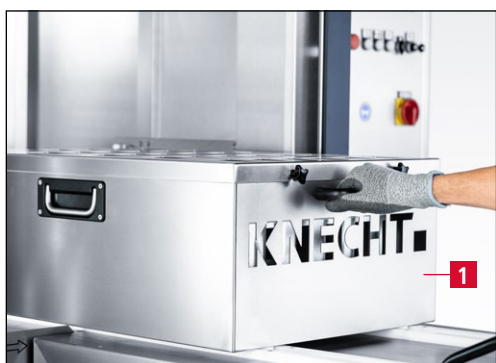
Figure 9-14 Moving an empty knife magazine into the machine
