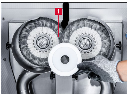
Figure 7-47 Removing the intermediate flange (7-47/1).
