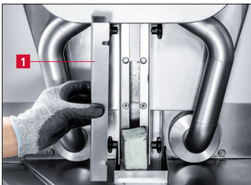
Figure 7-54 Removing the cover
