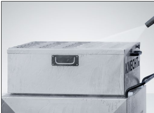
Figure 9-9 Cleaning the knife magazines
