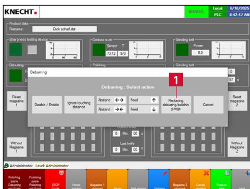
Figure 7-20 Deburring – Changing the deburring rings
