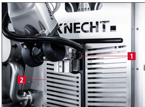
Figure 7-7 Removing the belt protection hood
