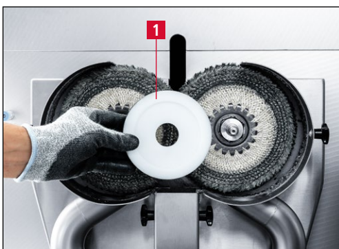
Figure 7-30 Removing the intermediate flange (7-30/1).
