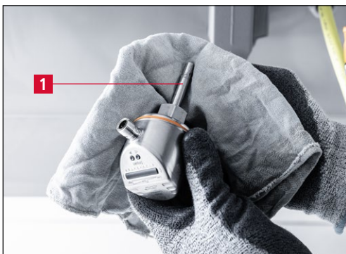
Figure 9-8 Cleaning the measuring probe
