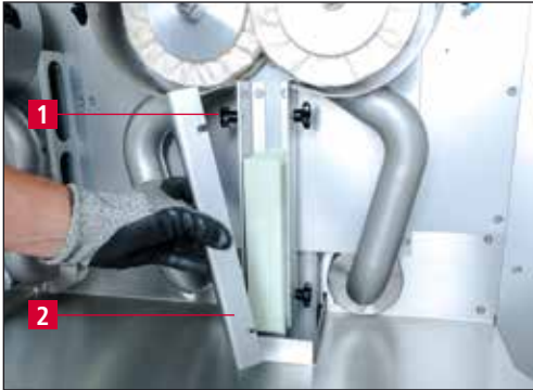
Figure 7-16 Changing the polishing paste
