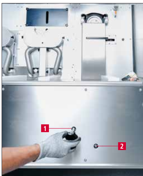
Figure 7-13 Aligning the wet-grinding belt
