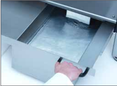
Figure 7-22 Changing the coolant
