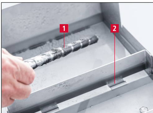
Figure 6-1 Inserting the magnetic bar
