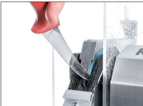
Figure 7-4 Sharpening hand knives
