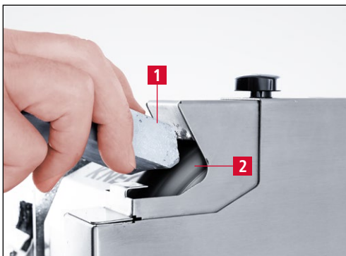
Figure 7-5 Applying the polishing paste
