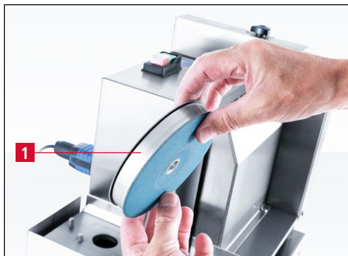
Figure 7-11 Mounting a new pair of grinding wheels
