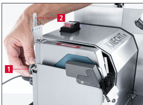
Figure 7-1 Setting the grinding angle
