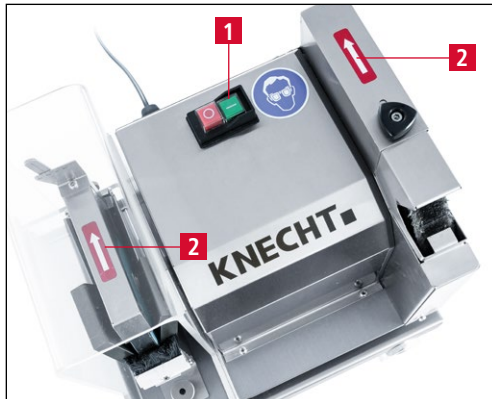
Figure 6-3 Checking rotating direction
