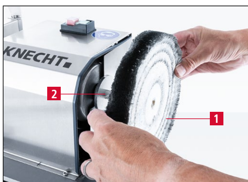
Figure 7-16 Replacing the polishing disk
