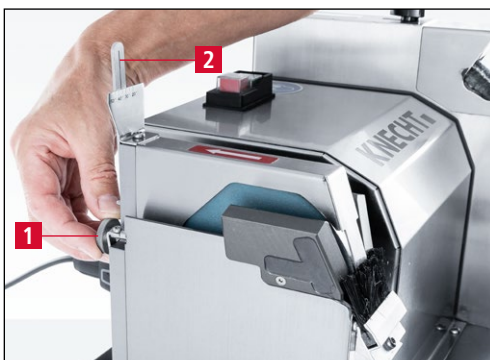
Figure 7-2 Setting the grinding angle
