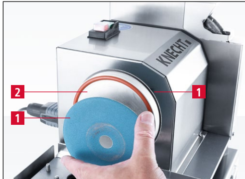
Figure 7-10 Removing the used grinding wheels
