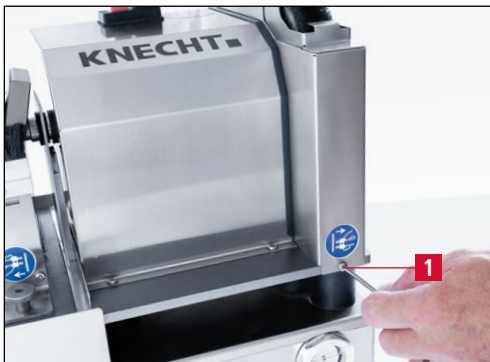
Figure 7-13 Loosening the polishing disk cover
