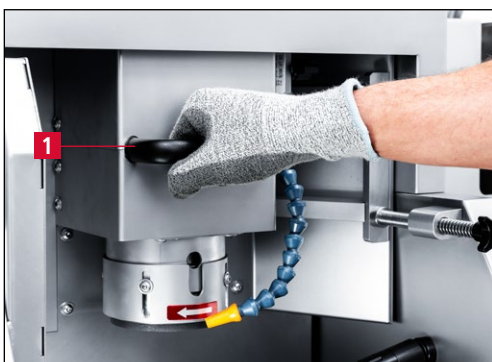
Figure 7-42 Moving the grinding unit to the working position
