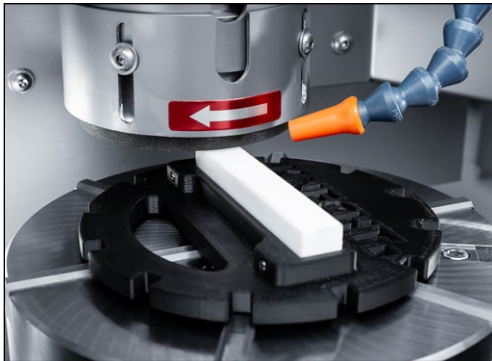
Figure 7-40 Grinding unit in working position
