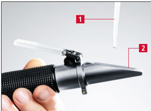
Figure 8-8 Measuring the cooling lubricant concentration
