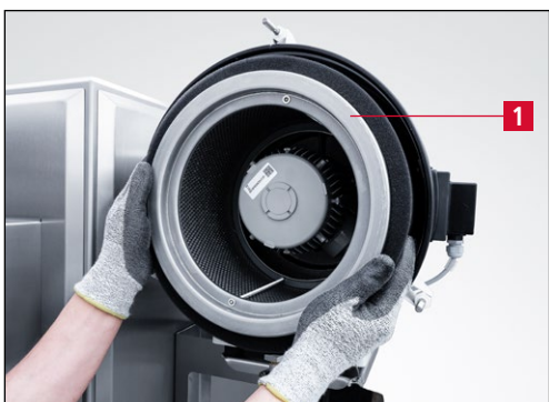
Figure 8-5 Removing the filter
