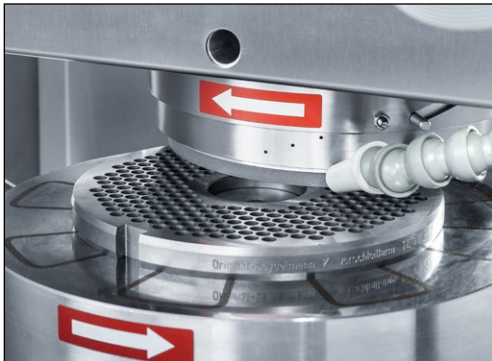
Figure 7-5 Rotary table in working position
