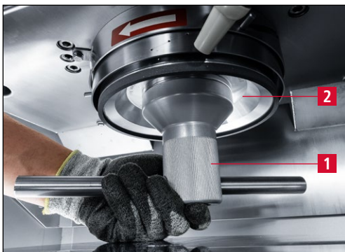
Figure 7-41 Loosening the grinding wheel
