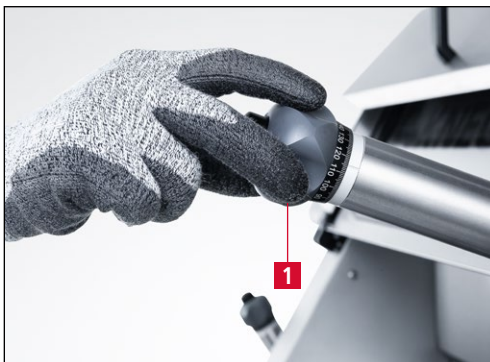
Figure 7-38 “Grinding unit” fine adjustment
