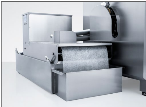
Figure 6-1 Filling the belt filter coolant unit
