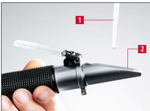
Figure 8-11 Measuring the cooling lubricant concentration
