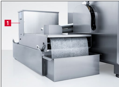
Figure 3-8 Belt filter coolant unit
