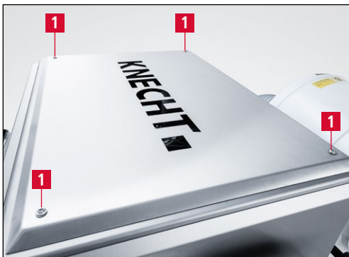
Figure 8-7 Opening the machine cover
