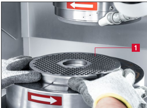
Figure 7-3 Placing the mincer plate on the rotary table
