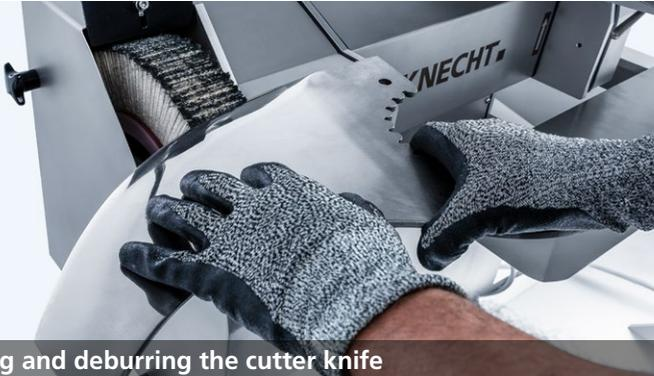
Polishing and deburring the cutter knife
