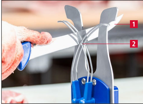
Figure 3-1 Honing the hand knife
