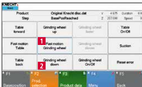
Figure 7-9 Dressing the grinding wheel
