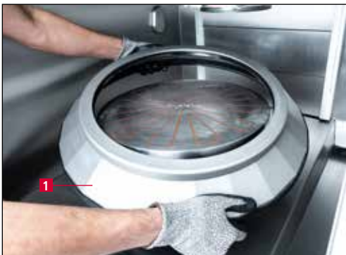
Figure 9-6 Removing the drip ring
