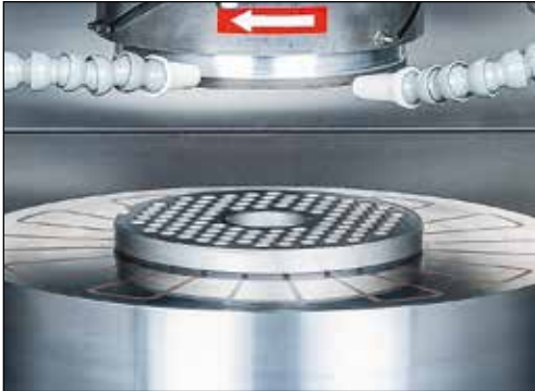
Figure 7-5 Mincing plate on rotary table
