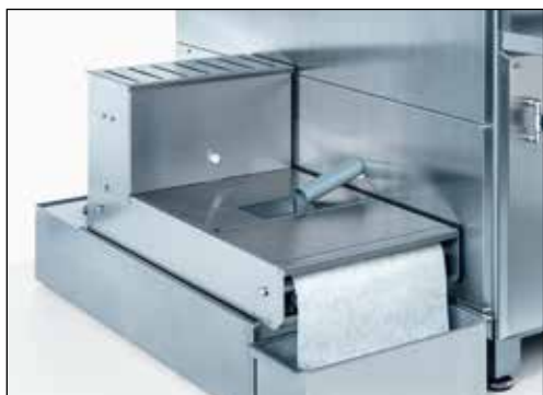
Figure 6-1 Filling the belt filter coolant unit
