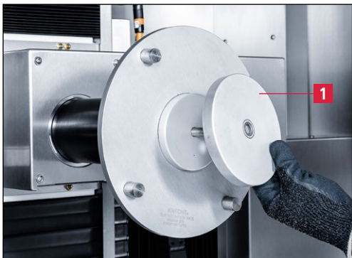
Figure 7-28 Retirer la bride de serrage
