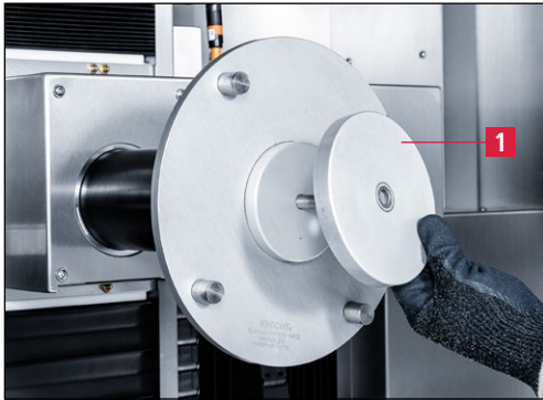
Figure 7-9 Retirer la bride de serrage
