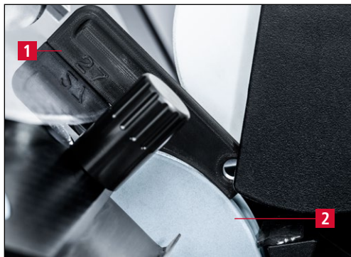
Figure 7-14 Setting the grinding angle
