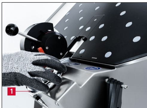
Figure 7-29 Moving the grinding unit to a middle position
