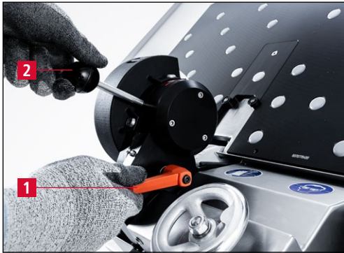
Figure 7-43 Swiveling the deburring wheel to the upper end position
