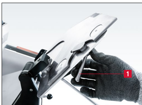
Figure 7-107 Locking the knife on the grinding plate
