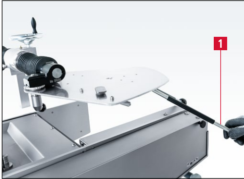
Figure 7-16 Swiveling the grinding plate backward
