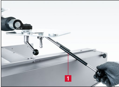
Figure 7-78 Swiveling the grinding plate to the rear
