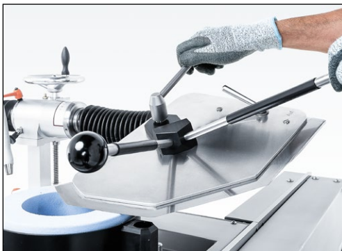
Figure 7-85 Aligning the knife on the grinding wheel
