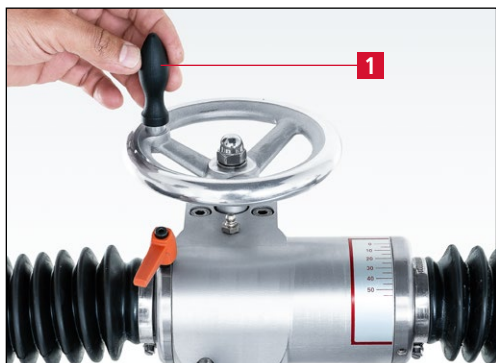
Figure 7-25 Reducing the grinding angle (convex grinding)
