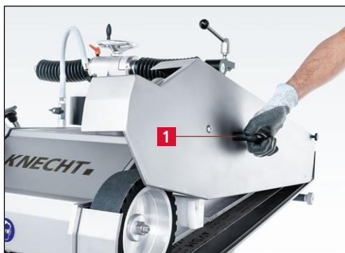
Figure 7-146 Opening the belt protection hood
