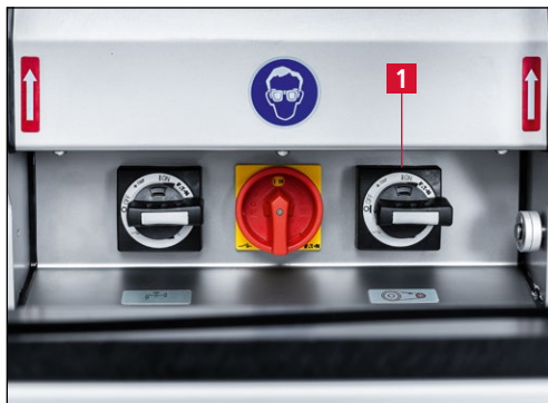
Figure 7-61 Switching on the grinding machine
