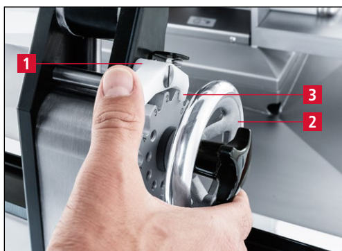
Figure 7-117 Bringing the grinding unit into grinding position "1"
