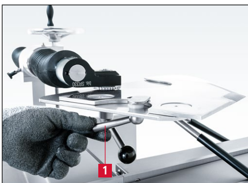
Figure 7-80 Locking the knife on the grinding plate
