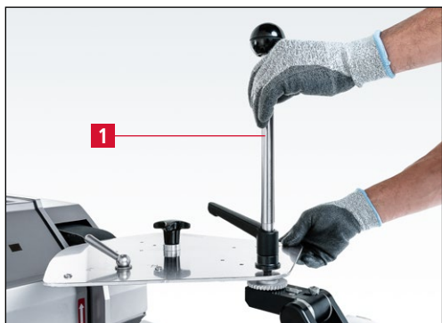
Figure 7-38 Slightly tightening the grinding lever
