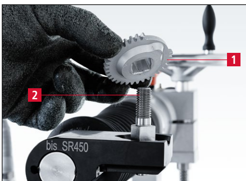
Figure 7-7 Inserting the function disc
