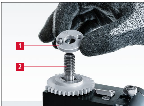
Figure 7-36 Setting the grinding angle
