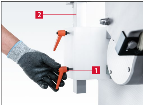
Figure 7-20 Adjusting the knife to the center of the grinding wheel
