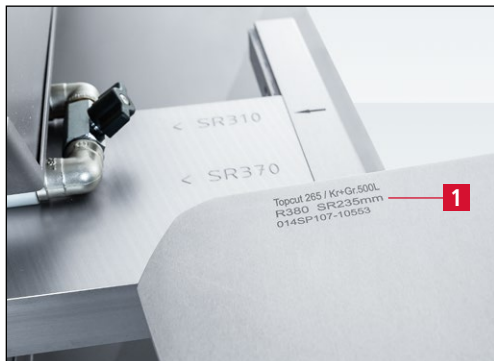
Figure 7-95 Displayed grinding radius on the SP 107 grinding plate
