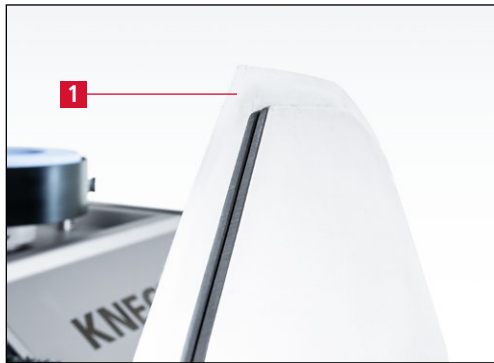
Figure 7-134 Checking the knife sharpness
