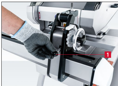
Figure 7-33 Locking the carriage in position
