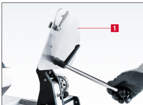
Figure 7-105 Swiveling the grinding plate backward
