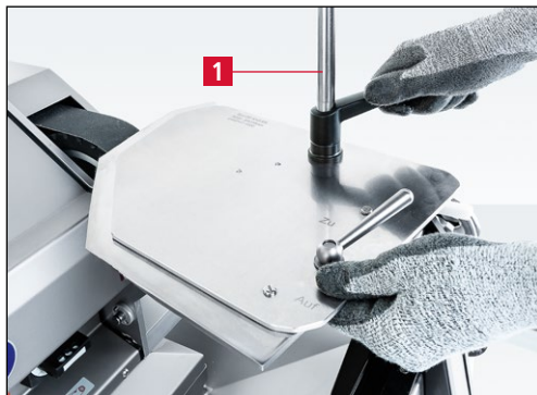
Figure 7-115 Tightening the grinding lever
