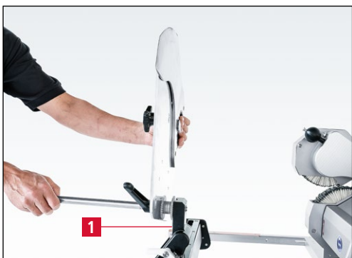
Figure 7-52 Cutter knife swiveled back and secured
