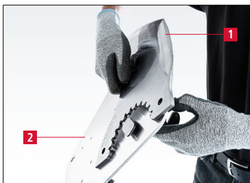
Figure 7-41 Clamping the knife onto the grinding plate
