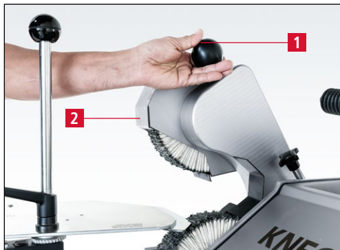
Figure 7-127 Swiveling the upper polishing unit upward
