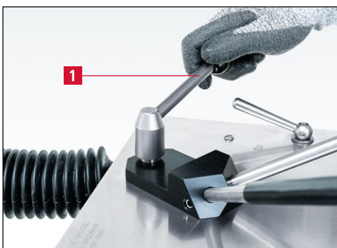
Figure 7-86 Tightening the clamping lever
