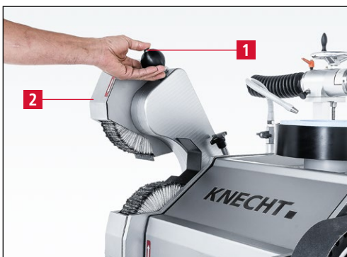
Figure 7-137 Upper polishing unit in rest position
