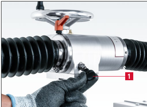
Figure 7-73 Engaging the locking bolt
