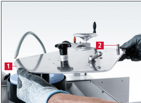
Figure 7-8 Mounting the grinding plate
