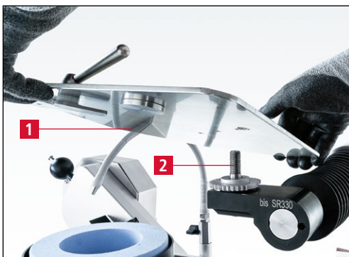
Figure 7-75 Mounting the grinding plate
