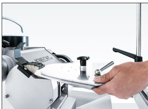
Figure 7-62 Polishing the knife bale
