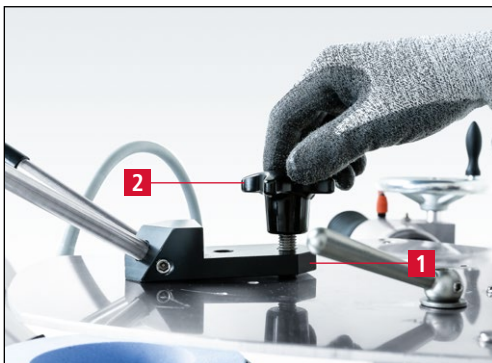
Figure 7-13 Mounting the grinding lever on the grinding plate
