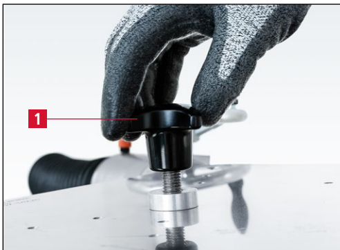
Figure 7-9 Removing the star handle
