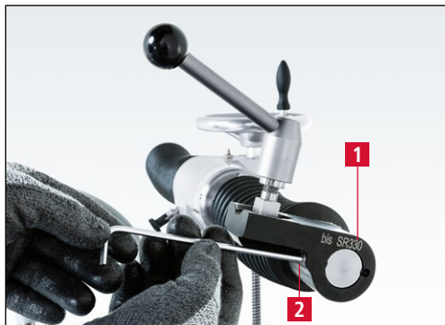
Figure 7-70 Fitting the mounting head
