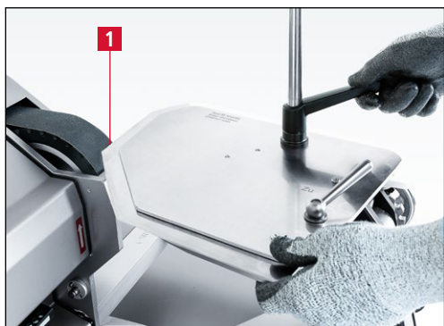
Figure 7-114 Aligning the knife on the grinding belt
