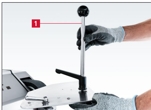
Figure 7-104 Clamping the grinding plate
