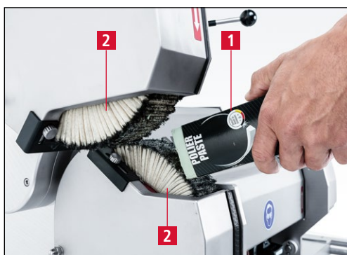
Figure 7-54 Applying the polishing paste
