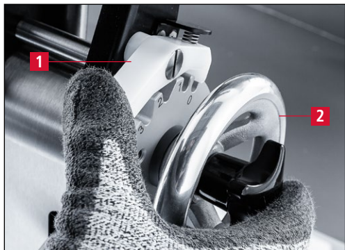
Figure 7-45 Bringing the grinding unit into adjustment position "0"
