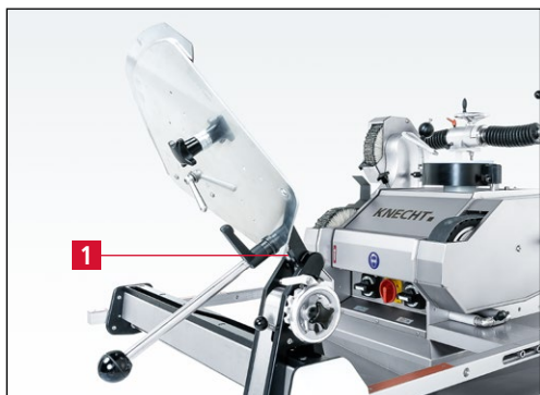
Figure 7-63 Knife outside the polishing area in secured position
