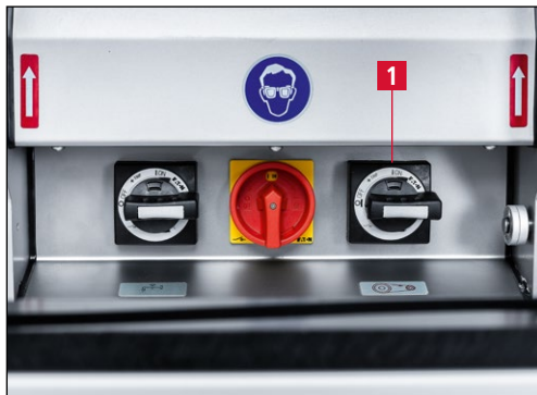
Figure 7-133 Switching off the grinding machine
