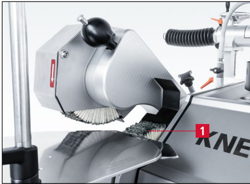
Figure 7-124 Knife rests on the finned brush
