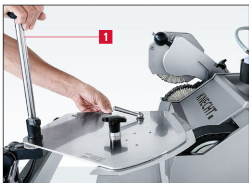
Figure 7-68 Swiveling the cutter knife to the next cutting segment and grind
