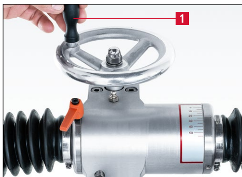
Figure 7-91 Reducing the grinding angle (convex grinding)
