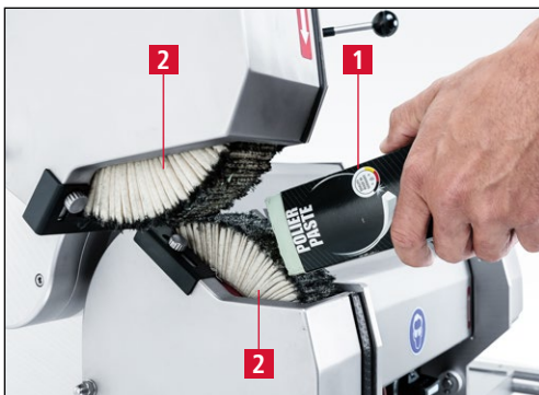
Figure 7-122 Applying the polishing paste
