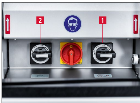
Figure 7-89 Switching on the grinding machine and coolant unit
