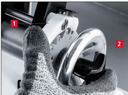
Figure 7-110 Bringing the grinding unit into adjustment position "0"
