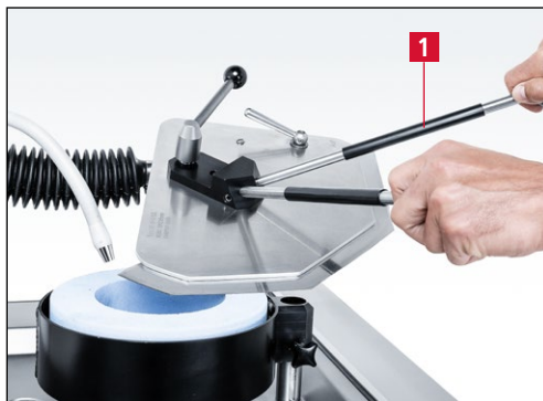
Figure 7-90 Grinding linear cutter knives
