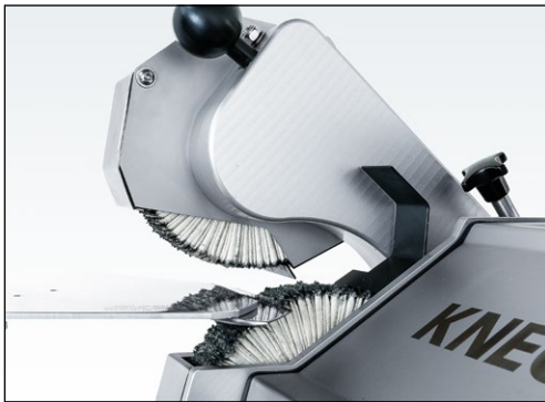
Figure 7-125 Distance between finned brushes approx. 20 mm
