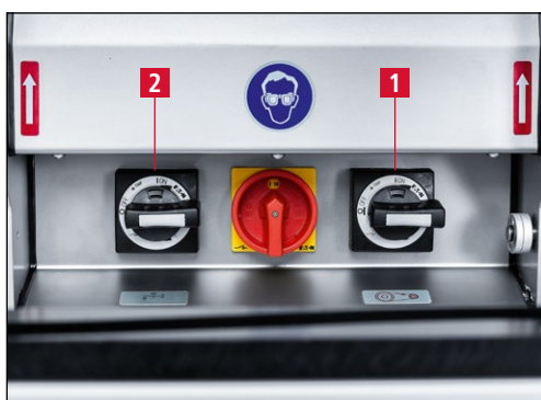
Figure 7-116 Switching on the grinding motor and coolant unit
