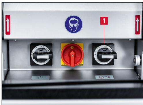
Figure 7-66 Switching off the grinding machine
