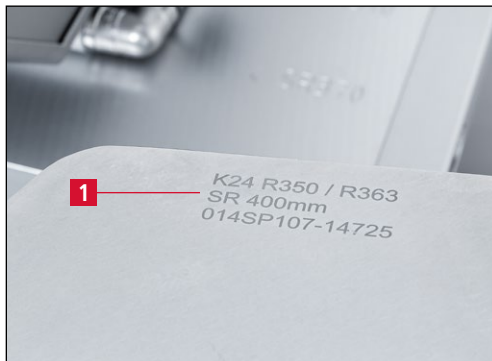
Figure 7-29 Displayed grinding radius on the SP 107 grinding plate
