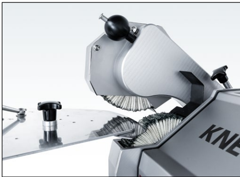
Figure 7-58 Distance between finned brushes approx. 20 mm
