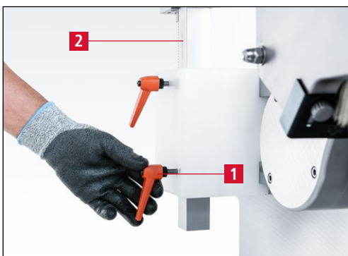
Figure 7-83 Adjusting the knife to the center of the grinding wheel
