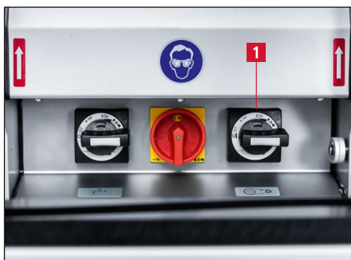
Figure 7-128 Switching on the grinding machine
