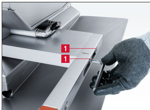
Figure 7-30 Loosen the M 10 screws
