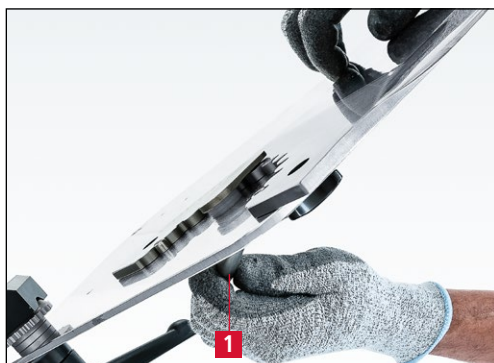
Figure 7-42 Locking the knife on the grinding plate
