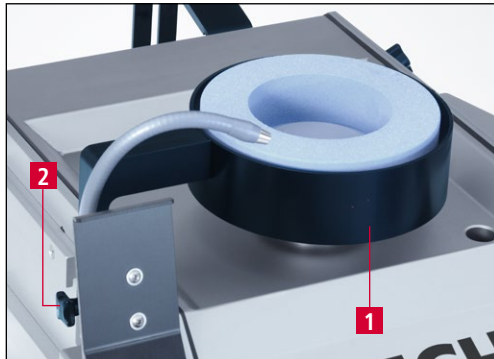
Figure 7-11 Adjusting the grinding wheel guard
