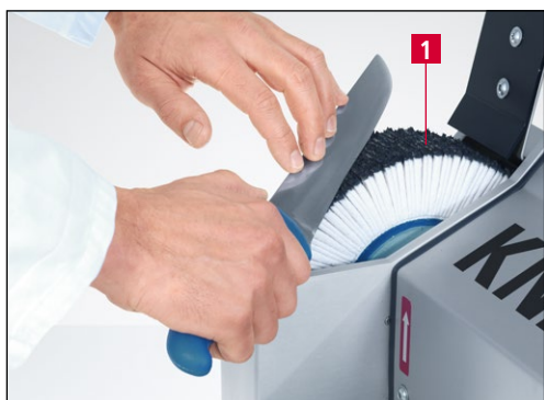
Figure 7-8 Deburring and polishing hand knives
