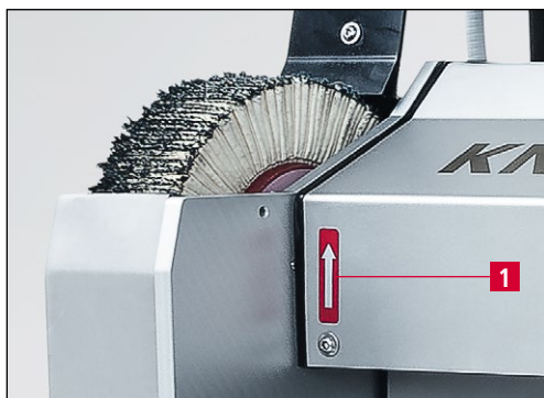
Figure 6-2 Checking the direction of rotation
