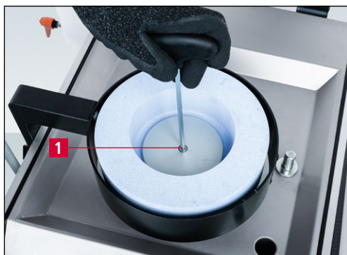
Figure 7-12 Replacing the grinding wheel
