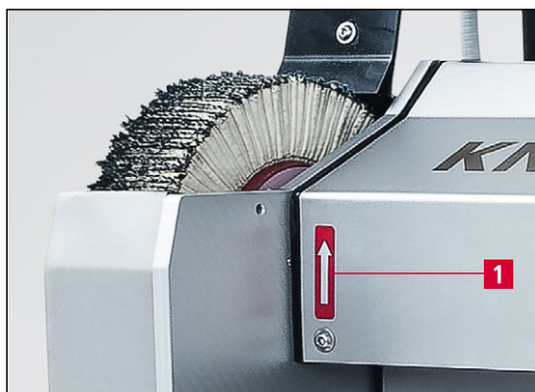
Figure 6-2 Checking the direction of rotation
