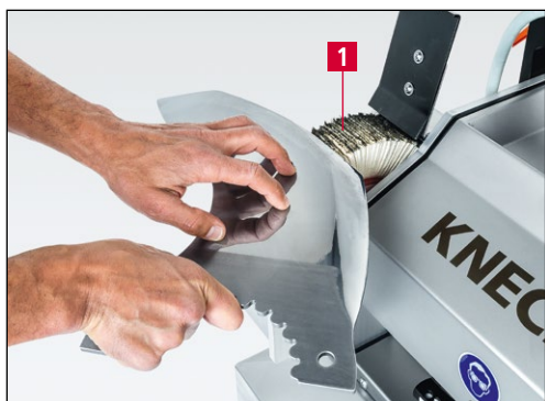
Figure 7-6 Deburring and polishing cutter knives
